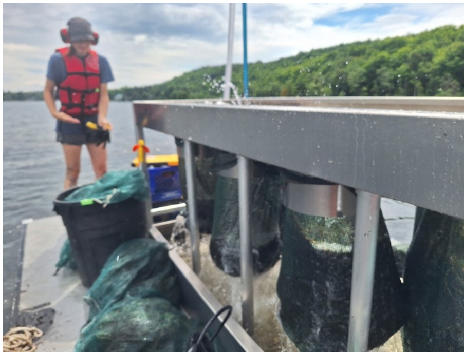
Figure9 : Table of the suction lift system used to bring the water milfoil to the surface.
